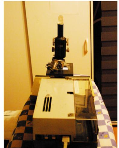
**Fig. 15. The microscope with the prism on top and the light source (slide projector).**
