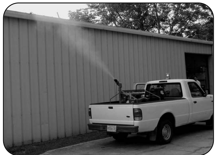
Figure 6. ULV applicator showing the fine mist as it leaves the nozzle.
